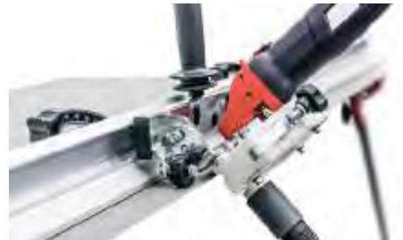
With a special beveling machine supported on a guide of suction cups and a sliding system on this by means of four adjustable nylon pulleys, offering total precision in the work.
