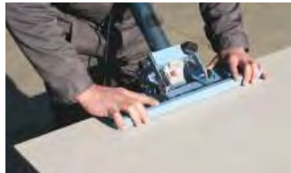
With a special beveling machine supported on the ARKLAM table using different abrasive discs depending on the type of finish that is required.
